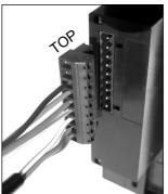
Installation of the protective cover after the electrical connection.
